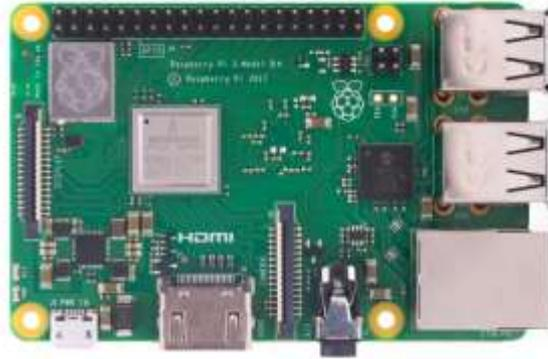
Gambar 2. Raspberry Pi 3 Model B+
