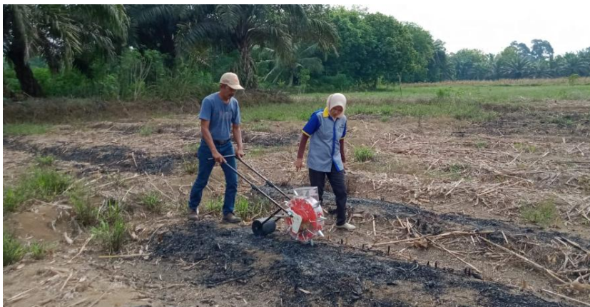
Figure 4. Rolling planter corn seeder trial
